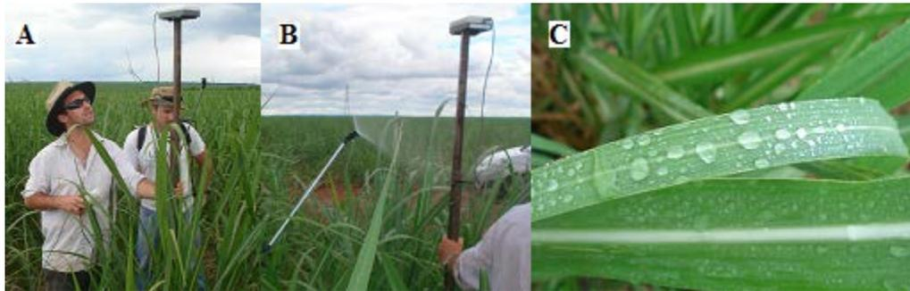
**Fig. 1. Collecting data with the sensor before (A) and during (B) the rainfall simulation; wet leaves after the rain simulation (C).**
